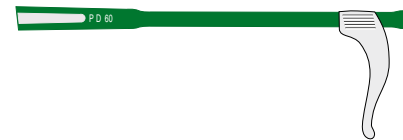
B Straight temple with adjustable length silicon hook.
